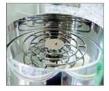
Recommended for measurements with d=0.01mg and wherever heavy air drafts occur.
