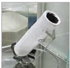
The holders are especially useful in course of weighing oval-shaped objects (bulbs, measuring vessels, test tubes etc.)
